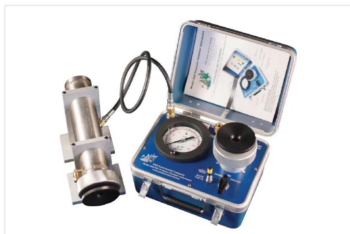
Figure 1: Scholander Pressure Chamber (Source: Pmsinstrumen)
