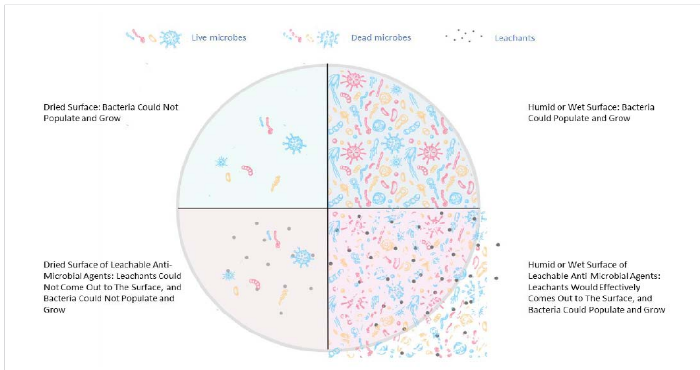
Figure 1: The living mechanism of bacteria on dry and wet surfaces of PP composites.
